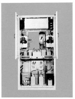
voltage supply feeds the modulator screen grids, as well as the plates and screen grids of the other RF and audio tubes. The bias supply provides voltages for the modulator, power amplifier and other biasing throughout the transmitter.
